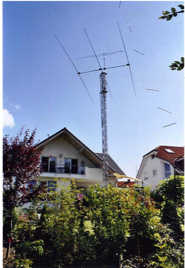
Fig. 7 – Vertical part of the „invisible antenna“ with the PVC insulators, including now also the 40m radiator.
